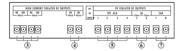
(3) 9V and 12V high-current output pairs. Each pair is an isolated output section providing up to 400mA.
